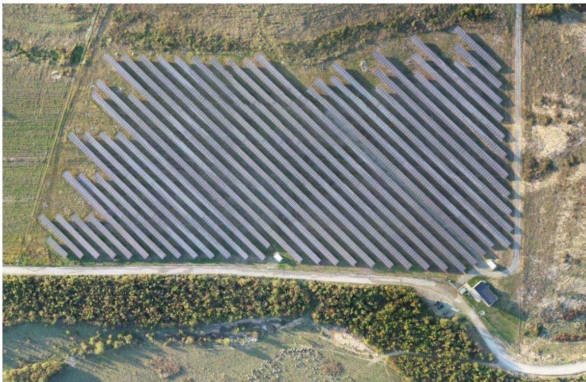
Figure 19 Eco Park, Madanaj- Kusar, Gjakovë, 3,000 kW Solar PV based on Feed-in Tariff
